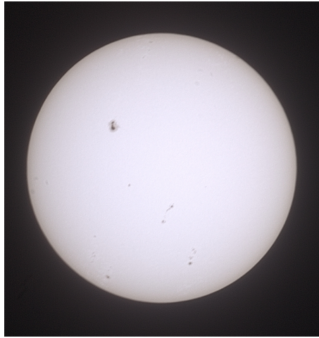
Figure 1: The solar white light image recorded at 10:00 UTC on July 11, 2023. The image was recorded using a Mylar filter and the 8 inch Newton telescope with a focal length of 1000 mm. Note the clear separation of the umbra and penumbra of the large sunspot. Students measured the limb-darkening effect in a radial profile.
