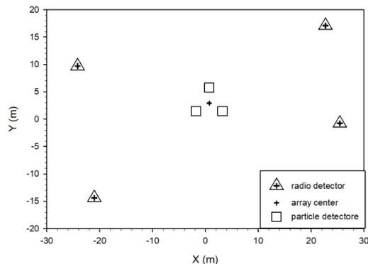
Figure 1: The SURA array. triangles show the current locations of the LPDA antennas and squares show particle detector for this study.
