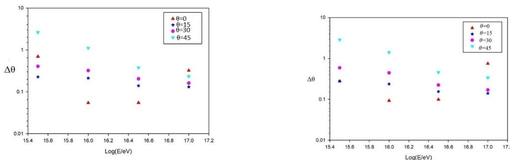
Figure 4: Error in the determinations of EAS arrival direction vs energy (right and left for triangular arrangement with sides of 5 and 10 meters, respectively).
