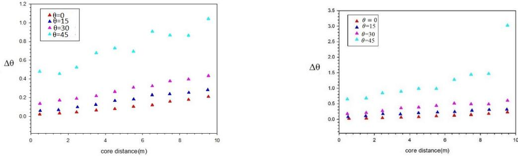
Figure 6: Errors in angular resolution vs core distances (right and left for equilateral triangular arrangement with sides of 5 and 10 meters, respectively).
