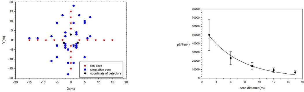
Figure 5: Left A simulated core position. The geometry is similar to that of the SURA array. Right The particle density as a function of the distance from the shower axis for the event shown on the left.
