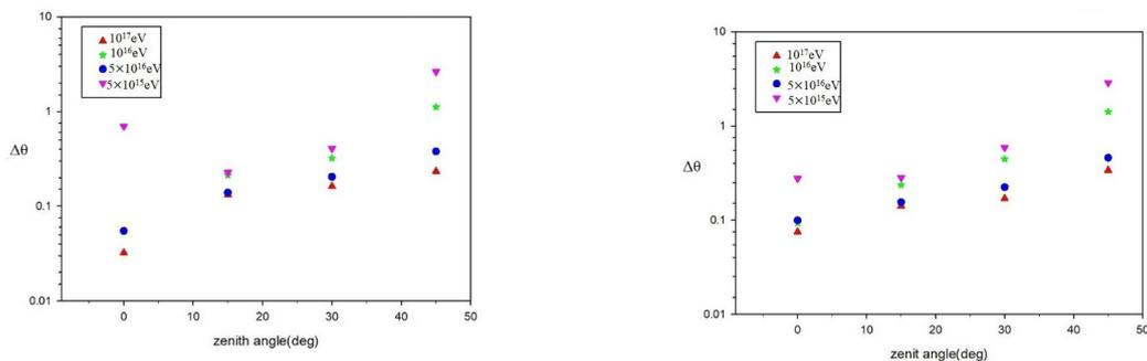
Figure 3: Error in the determinations of EAS arrival direction vs zenith angle (right and left for equilateral triangular arrangement with sides of 5 and 10 meters, respectively).
